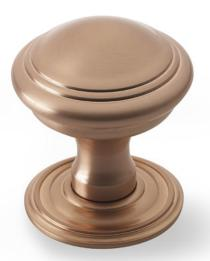
Sateen polished, pure copper plating on top of a satin finish solid brass surface, with a high performance electrophoretic lacquer protection. Electrophoretic lacquer offers superior adhesion, durability and corrosion resistance over conventional lacquers.
